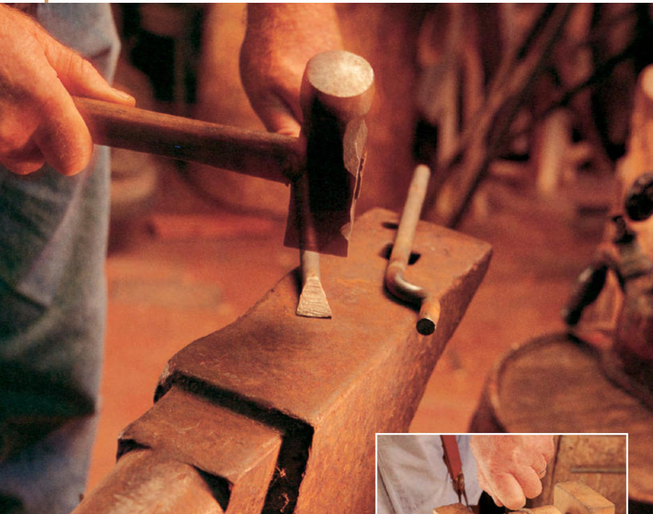
The drive center is shown here being formed, with the jigsaw crankshaft lying next to it. After rough shaping, the center is filed and ultimately takes on its spade-bit shape. The center is then mounted in the drive pulley by tightening the stop collars.
